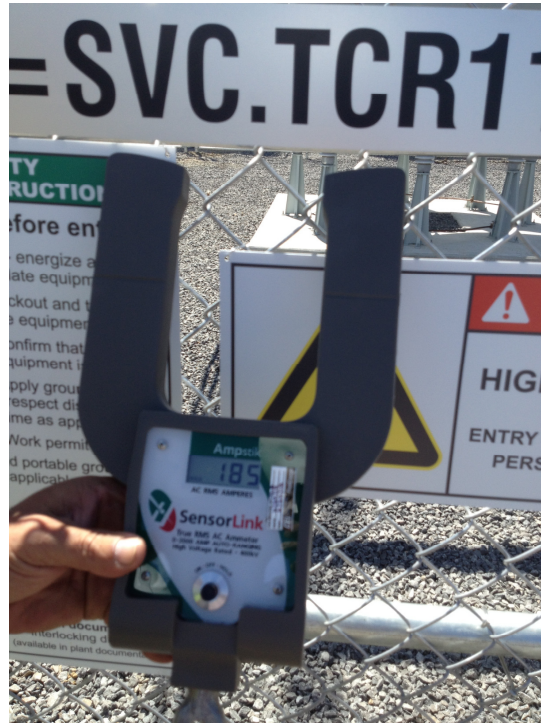
Figure 1: High Current in the TCR Branch Fence
