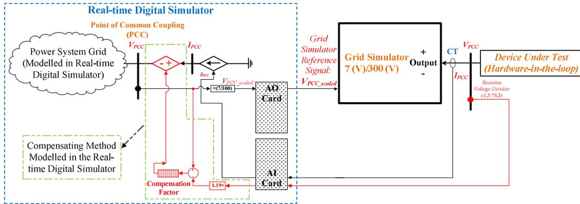
Fig. 1: Block diagram of a typical PHIL testing [1]-[15]
