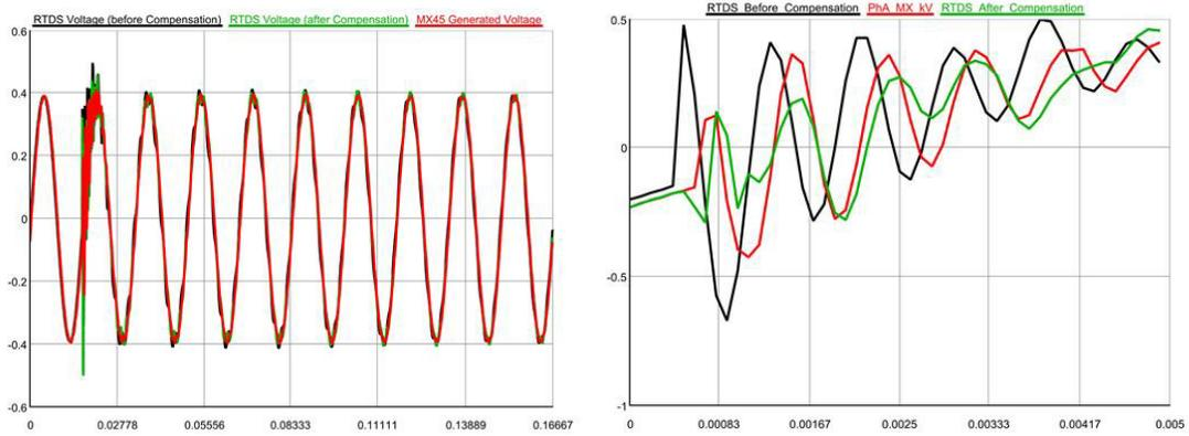
HIL Voltage (kV); black: simulated voltage in the real-time digital simulator before compensation, green: simulated voltage in the real-time digital simulator after compensation, red: generated voltage by grid simulator
