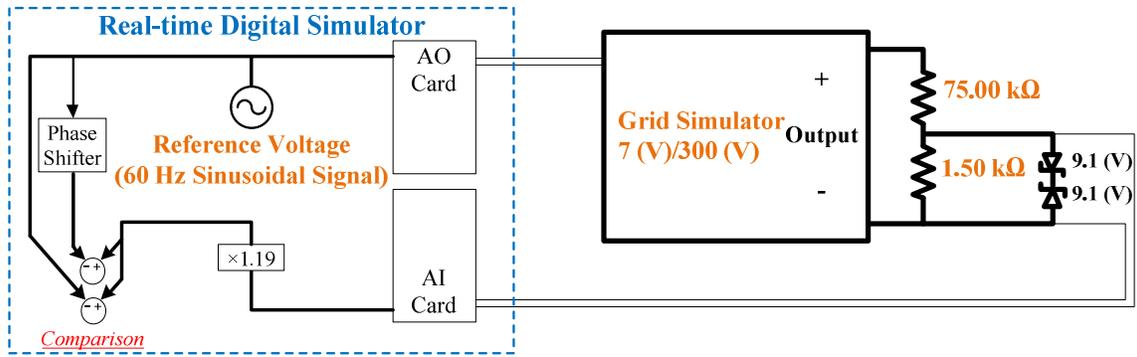
Fig. 4: Circuit configuration for testing generated delay by grid simulator in the typical real-time simulation and PHIL test.
