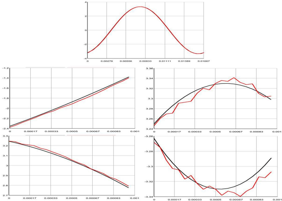
Fig. 3: Test results of delay generated by AI/AO cards; Black: Voltage Sent out by AO Card, Red: Voltage Received by AI Card
