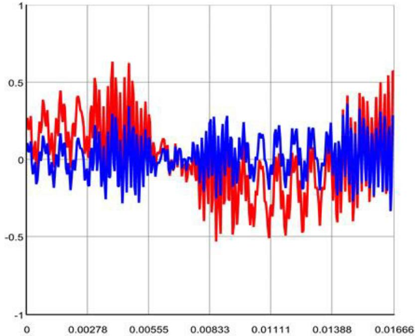
Fig. 6: Test results of error signal after shifting phase; Red: error signal generated by subtracting reference voltage sent out by real-time digital simulator and scaled back grid simulator voltage, Blue: error signal generated by subtracting  $3.456^\circ$  shifted reference voltage sent out by real-time digital simulator and scaled back grid simulator voltage.
