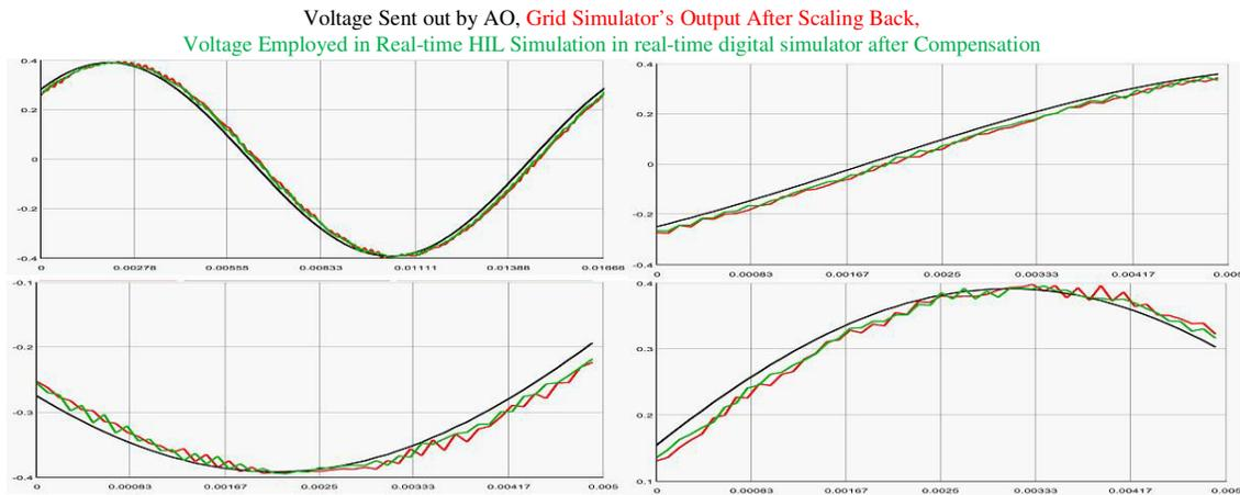
Fig. 8: Voltage employed in PHIL simulation; Black: voltage sent out by AO Card, **Red: Grid Simulator's output after scaling back**, **Green: voltage employed in real-time PHIL simulation in real-time digital simulator after compensation.**
