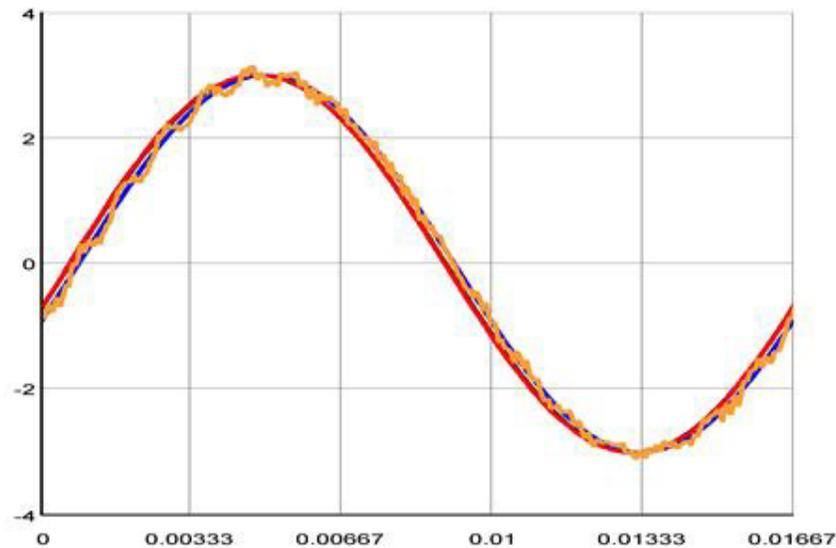
Fig. 5: Test results of delay generated by grid simulator; Red: reference voltage sent out by real-time digital simulator, Blue: reference voltage shifted by  $3.456^\circ$  and sent out by real-time digital simulator, Orange: voltage generated by grid simulator.
